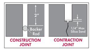
Do not use compressible backer rod in saw cut contraction/control joints less than 2" deep. Compressible rod may be used as a base in construction joints if placed 2" below floor surface.
